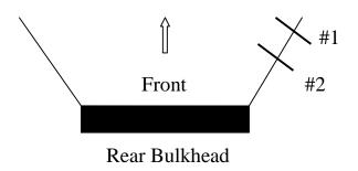
For extremely bumpy conditions the car will handle best with no sway bars. This will allow the car to soak up the big bumps easier.
