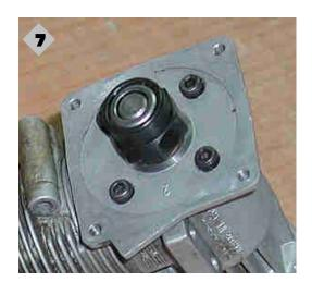
Add lightweight oil inside the space occupied by the axle until the space is full. Rotate the axle head several times so the oil lubricates the bearing.
