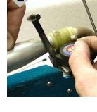
Move the pull start handle to the other side of the pipe as shown.
