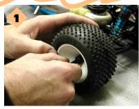
Use your wheel nut wrench to remove the nut from the rear wheel next to the engine. Remove the wheel.
