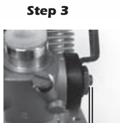
Low Speed Mixture: 1/16" of screw showing (1.5 mm)
