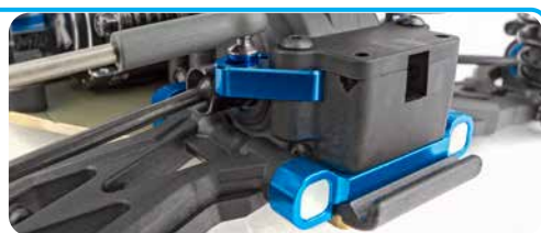
New 22.5 kickup and bulkhead options. T6.4 offers: 20.0, 22.5 and 25.0. T6.2 offers: 25.0 and 30.0.
