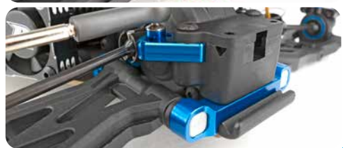
Updated CVA driveshafts, C and D mounts. T6.4 offers: 92.5mm shafts and wide C and D mounts. T6.2 offers: 91mm shafts and narrow C and D mounts.
