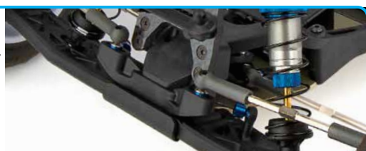
Updated CVA driveshafts, C and D mounts. T6.4 offers: 92.5mm shafts and wide C and D mounts. T6.2 offers: 91mm shafts and narrow C and D mounts.
