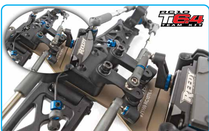
New adjustable height steering system. T6.2 is not adjustable
