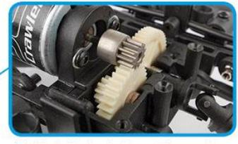
13.98:1 Ratio 3-Gear Transmission with Integrated Motor Mount
