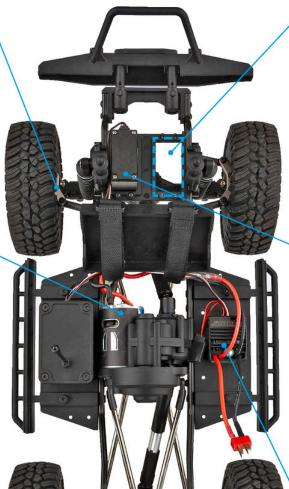
INTEGRATED SERVO WINCH MOUNT: Mounting a winch directly to the chassis is the strongest and most reliable spot on any trail rig. Positioned alongside the steering servo for overall chassis balance and weight distribution.
