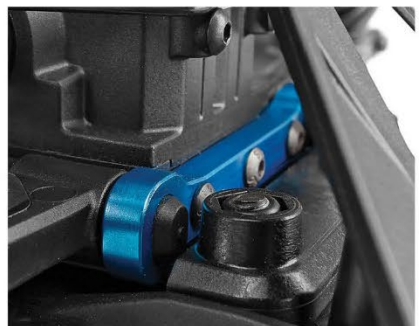
Aluminum arm mounts with adjustable toe, kickup and anti-squat.
