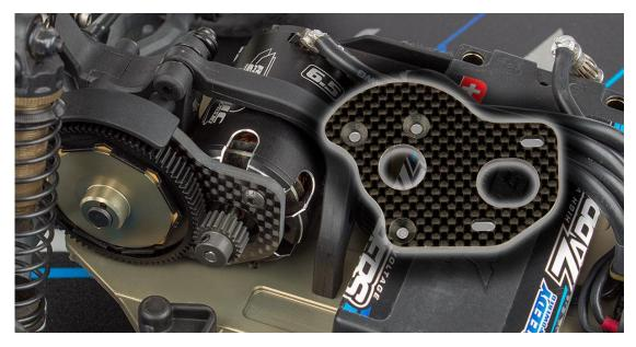
Our new Factory Team Motor Plate adds strength and rigidity with its 3mm thick material, while also reducing the weight by 40% over the stock motor plate. It fits the Laydown and Layback gearboxes on the B6.1, B6.1D, T6.1, and SC6.1.
