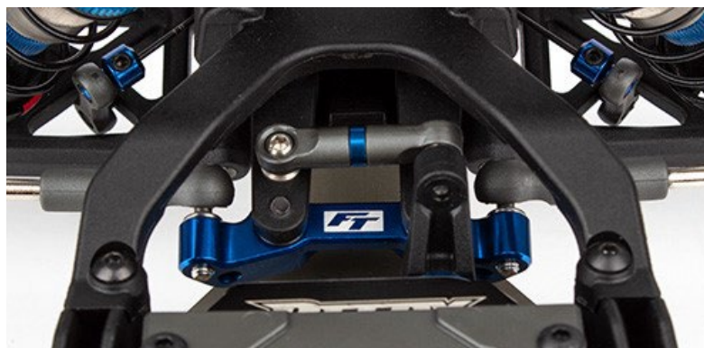
#91984 Steering Rack mounted in the RC10B6.4
