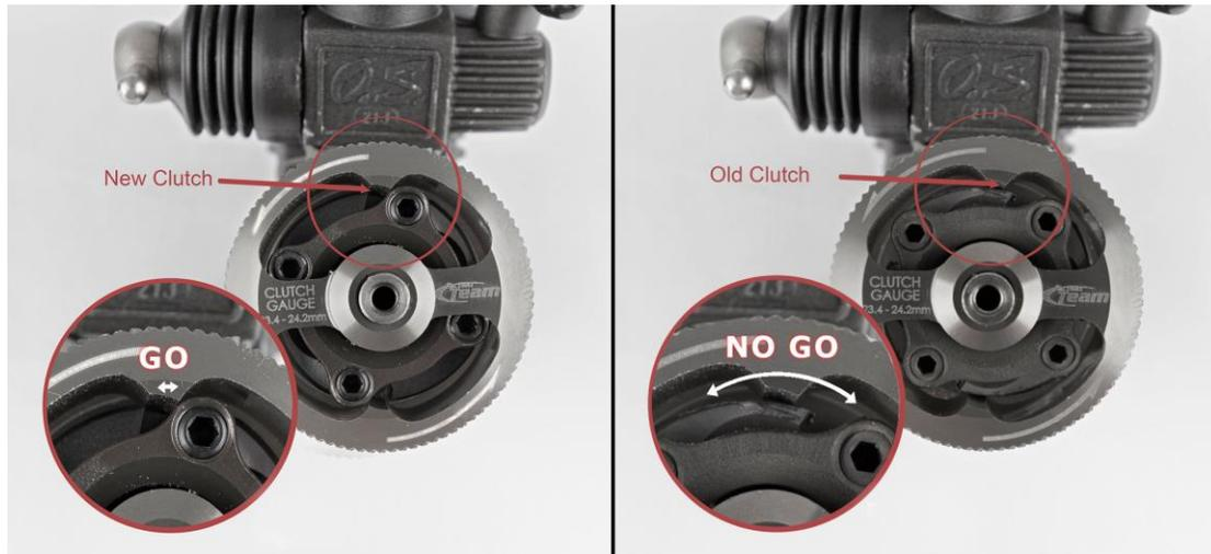
Worn-out clutch shoes can negatively impact the performance of the clutch and cause an engine to intermittently flame out even when tuned properly. This decreases a vehicle's overall performance and can cause headaches at the track.
