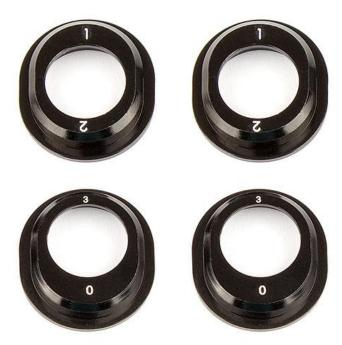
Replace your standard diff height adjusters with these long-lasting aluminum versions. Orientation numbers are etched onto the inserts, making them easy to read. Compatible with RC10B6.1, RC10B6.1D, RC10B6.1 FL, RC10T6.1, and RC10SC6.1
