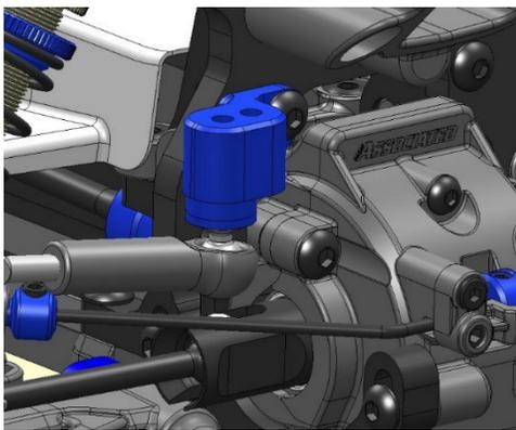
The intent of these mounts is to allow drivers more versatility than what is available on the kit tower, particularly regarding mounting the inner rear ballstud, which affects the roll center and camber gain of the car. The extent of the available adjustment range will depend on multiple factors such as differential height, hub height, link length, and more.
