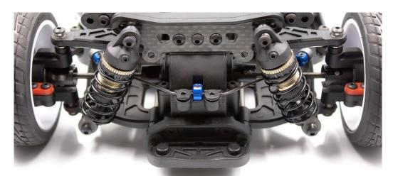
(Pictured: Shock and anti-roll bar sets installed on the Apex2.)
