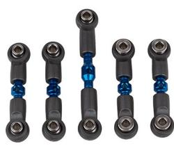
Made for the Apex2 and Apex2 Sport chassis, this turnbuckle set allows the vehicles' front and rear toe angle to be adjusted. Toe angle can affect how the car performs. Whether it's increasing stability, reducing oversteer, or mitigating issues related to understeer, the ability to adjust toe angle allows a definite improvement in performance.
