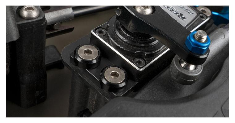
Gain more secure servo mounting with these aluminum servo washers. They preserve the structural integrity of the servo ears.
