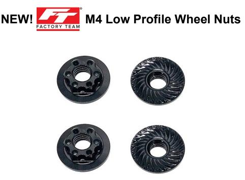
The Factory Team M4 Low Profile Wheel Nut is designed to fit on the front of car models (example: B74, B64, TLR 22, TLR 22-4, Tekno EB410, Yokomo YZ-4 SF) that require a thin nut to maintain the legal width limit at major events. With large diameter locking serrations, these wheel nuts "bite" into the face of the wheel to create a secure hold.
