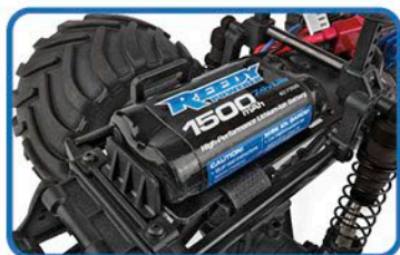
1500mAh Li-Ion 7.4V 2-cell battery and charger
