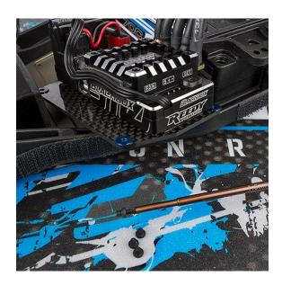
This #91754 ESC plate is a Factory Team lightweight option that provides for easy installation and removal of electronics for chassis cleanup.
