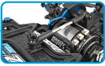
Rod end battery brace parts and hardware included in kit
