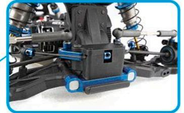
Front and rear anti-roll bars to provide less body-roll and more traction on high-grip surfaces
