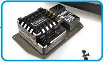
Steel electronics and under-servo weights for improved balance and lower overall center of mass
