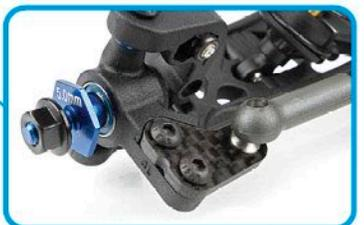
Bolt-on +1 carbon fiber steering arms for improved steering response
