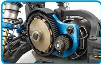
Octalock spur gear and 11mm Octalock LCF pads utilizing the heavier B74.1 slipper spring
