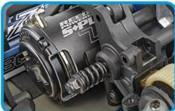
Lightweight aluminum one-piece top shaft and gear
