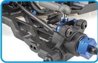
New rear hub assembly with modular vertical ball stud camber link mount and axle height adjustment
