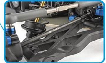
67mm CVA bones for reduced bone plunge and minimized friction at drive pin
