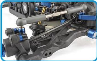
New symmetric 73mm rear arms with improved geometry and stiffness can be flipped to allow an in-between rear shock mounting position
