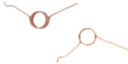
fig. 1 Motor springs. When the two ends are in a straight line rather than angled, tension is greater.
