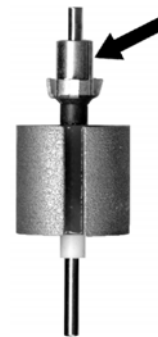
fig. 2 The arrow points to the commutator portion of the armature.
