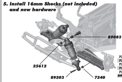
If you are upgrading from a small bore shock to the larger #7262 16mm shock, you will need #7263 16mm Shock Kit Mounting Hardware and 16mm Shock Springs. (Parts for steps 3-4 are found in #7263.)
