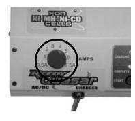
Turn the knob to set the charge rate in amps.
