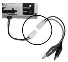
When using the alligator clip adapter, connect the red to the positive on the battery pack and black to the negative.
