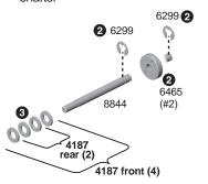
Slide the VC foam/ bobbin assembly over the #8844 shaft and then two #5407 O-rings. Place a couple drops of oil on the O-rings.
