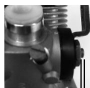
Low Speed Mixture: 1/16" of screw showing (1.5mm)
