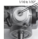
Idle Speed: 1/32" to 1/16" opening (.8 to 1.6 mm). Larger opening = higher idle speed. Smaller opening = lower idle speed.
