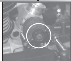
Low Speed Mixture: 4 1/2 turns out at full throttle Clockwise = Leaner Counterclockwise = Richer
