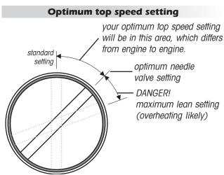
gine to run at full speed. Run your car two or three passes at full throttle and note its performance. Turn the high-speed mixture screw clockwise 1/8 of a turn and retest your car, again noting the vehicle's performance. Continue to lean the mixture and retest the vehicle until the highest speed is achieved. At that point, turn the mixture screw counterclockwise 1/16 of a turn. This is the optimum setting that the engine should be set to run at.
