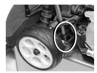
**5** With chassis lined up like step #2 and front posts already set, unscrew and slide the rear posts located on the rear platform so that they are pinching the rear of the chassis loosely.
