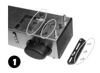
**2** Remove the case end and starter bulkhead.
