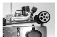
**3** With the chassis lined up like step #2, adjust the spring-loaded platform to support the rear of the chassis. The spring-loaded platform can be flipped to accommodate the length of the chassis. If needed, disassemble, turn the platform 180 degrees, and reassemble.
