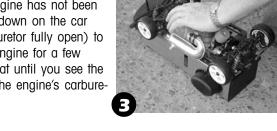
**4** Make sure the radio is on and you have full control of the carburetor/throttle.
