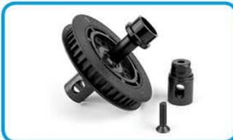
Front spool with replaceable hardened steel outdrives. Hardened steel surface for minimum wear. CVA bone blade is no longer necessary, eliminating failure of the blade under impact.
