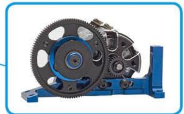
One-piece motor mount. Central mounting to allow free chassis flex in either direction. One-piece design ensures proper spur/pinion gear alignment.
