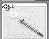
Snap e-clip into groove on shock shaft. Install piston onto shaft, and snap second e-clip into groove on shock shaft.
