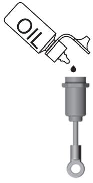
2 Slowly move the shaft up and down several times to allow air bubbles to escape to the top.
