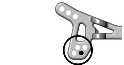
**ACKERMAN** is a term describing the effect of the inside front wheel turning tighter than the outside front wheel. The standard setup works best in most conditions and is preferred by most of our Team drivers.
