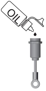
4 Push the shaft up until the piston is level with the top of the body. The oil will bulge up above the shock body.
