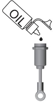
9 If the shock rebounds too fast, or you cannot push the shaft in until the eyelet hits the body, there is too much oil. Loosen the cap about a full turn and pump out a small amount of oil by pushing the shaft in. Retighten the cap and try steps 6-7 again.
