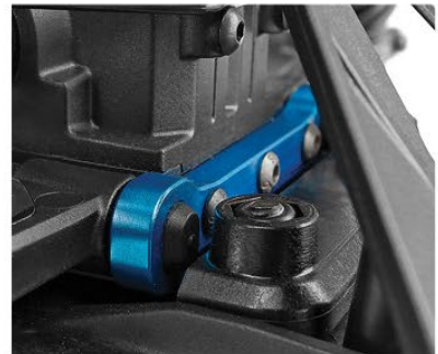
Aluminum arm mounts with adjustable toe, kickup and anti-squat.
