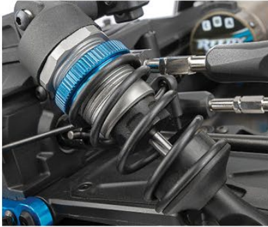
Threaded, aluminum oil-filled shocks with adjustable positions.
