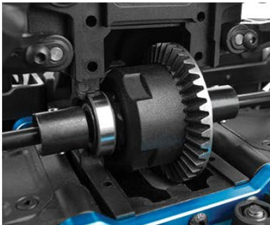
Oil-filled front, center, and rear differentials with steel ring and pinion gears.
