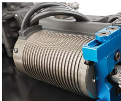
Reedy SC1500-BLC brushless ESC and high-power Reedy 685-SL4 2100kV brushless motor are 4S-6S compatible.
