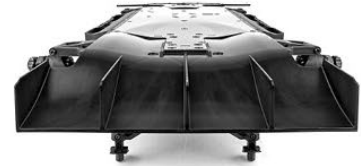
A rigid, die-formed aluminum chassis with integrated splitter and diffuser for superior aerodynamics at high speeds.
