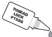
This symbol indicates where Thread Lock Adhesive should be applied. \*not included
