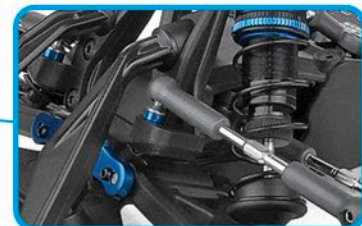
Vertical ball ends for roll center adjustments, front and rear
