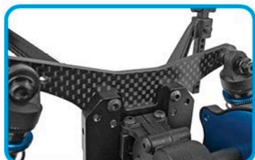
Updated mid-motor rear carbon fiber shock tower for oval
