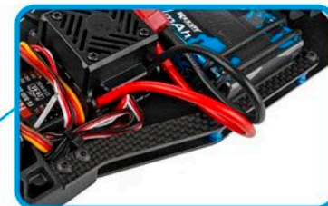
New carbon fiber chassis side braces
