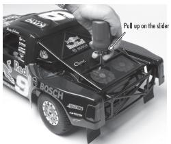
Insert the glow igniter into the remote glow plug. Make sure it 'grabs' the glow plug.
