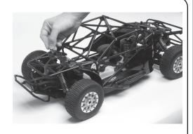
Attach roll cage to chassis with the supplied body clips.
