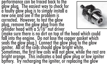
**Flooding.** Symptoms of a flooded engine include difficulty in starting, muffled sounds coming from the exhaust, Pro-Start won't operate, and excess fuel draining from the exhaust outlet. Remove the glow plug with a 5/16" nut driver. Tilt the buggy on its side and run the Pro-Start pistol a couple of times to pump the excess fuel out of the engine. Re-install the glow plug and try starting again.
