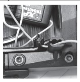
Trim the antenna tube to fit the amount of antenna wire that will be sticking out of the receiver box before installation!
