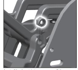
Install locknut into groove of the rear bumper brace (lower). Then screw in the 4-40x1 3/4 shcs until snug.
