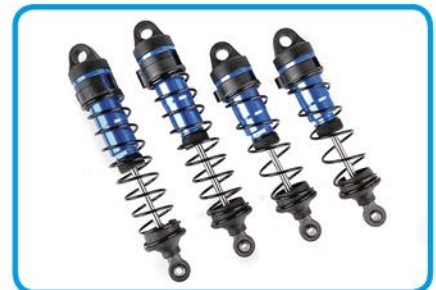
Fluid-filled, blue anodized aluminum V2 12mm shock bodies, front and rear
