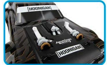
Injection-molded hood, turbo and exhaust accessories
