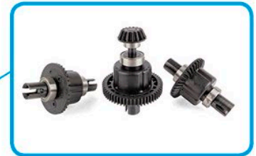
Three sealed differentials
