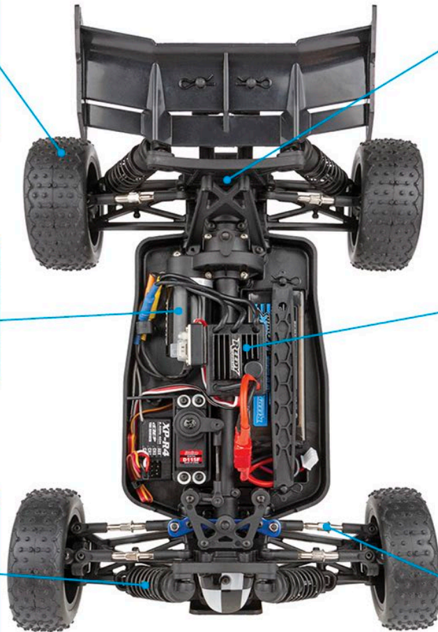
Three sealed differentials
