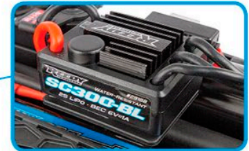
Water-resistant high-power Reedy brushless speed control
