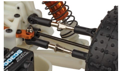
Turnbuckles to adjust camber and toe
