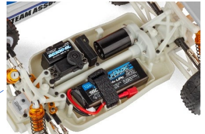
Molded tub chassis with covered center driveshaft
