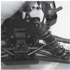
**Step 2:** Finish installing the shock to the standoff. Set your vehicle to your desired droop setting. To increase your droop turn the droop screw (from the top) counter-clockwise (loosen), turn the droop screw (from the top) clockwise (tighten) to decrease your droop. Remember, never back the screw out beyond full droop or you could risk damage to your vehicle.
