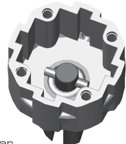
Align pin with groove in sun gear
