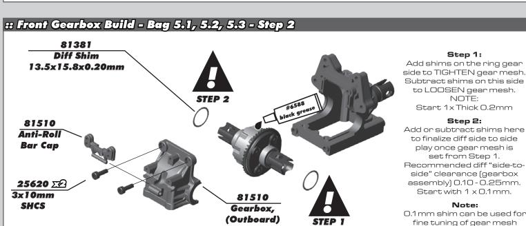
side to TIGHTEN gear mesh. Subtract shims on this side to LOOSEN gear mesh. NOTE:
