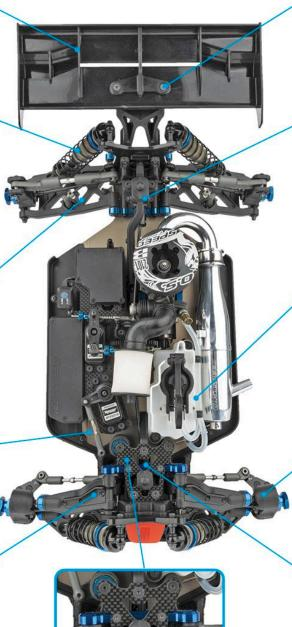
Carbon fiber front top plate centralizes the front chassis brace for balanced flex in all directions
