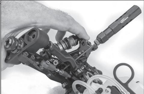
**Front Droop:** Increasing front droop (loosen droop screws) will increase off-throttle steering. It also allows the front end to lift more, giving more rear grip and less front grip on-power. Remember to never loosen the screws beyond the FULL DROOP setting. Decreasing front droop (tighten droop screws) yields more on-power steering and quicker response at the expense of some stability in bumpy sections. It will also give less off-throttle steering.
