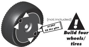
When gluing tires to wheels, use a fast-curing tire glue (CA) (AE # 1597). This is available at your local hobby shop. Make sure to clean the mounting surface of the tire and wheel with alchohol for best adhesion.
